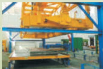
Fully Automated Concrete Placing & Finishing equipment
