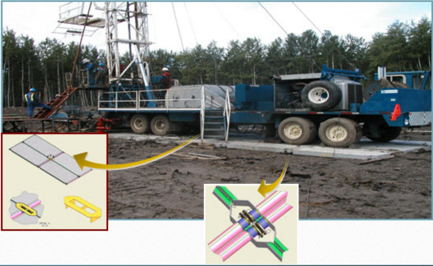
AN ADVANCED VERSION OF THE ENVIROMAT CAN WITHSTAND 40 TONS OF DYNAMIC LOADING!
