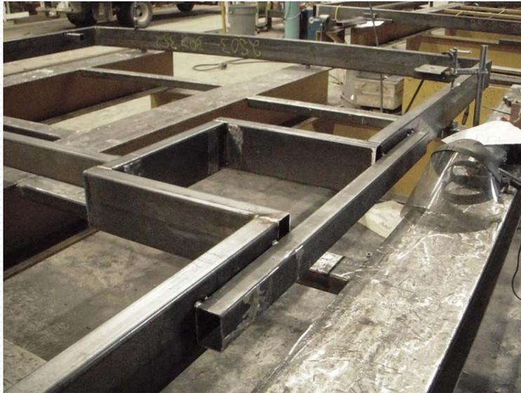
**INTRICATE FRAMING WITH TEMPORARY BRACING TO MINIMIZE WARPING EFFECT DUE TO WELDING WHICH WILL BE SIGNIFICANTLY ELIMINATED WITH THE AUTOMATED WELDING AND JIGGING SYSTEM UNDER CONSIDERATION**
