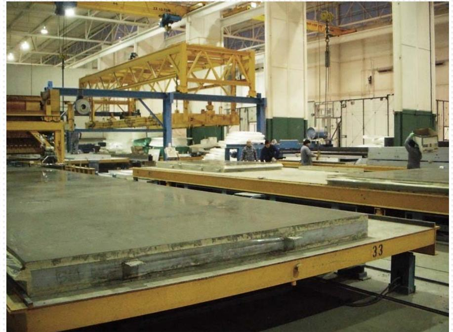
**FRESHLY POURED AND FINISHED CONCRETE PANELS AT THE CENTRAL PORTION OF THE IHI R&D AND MANUFACTURING FACILITY**
