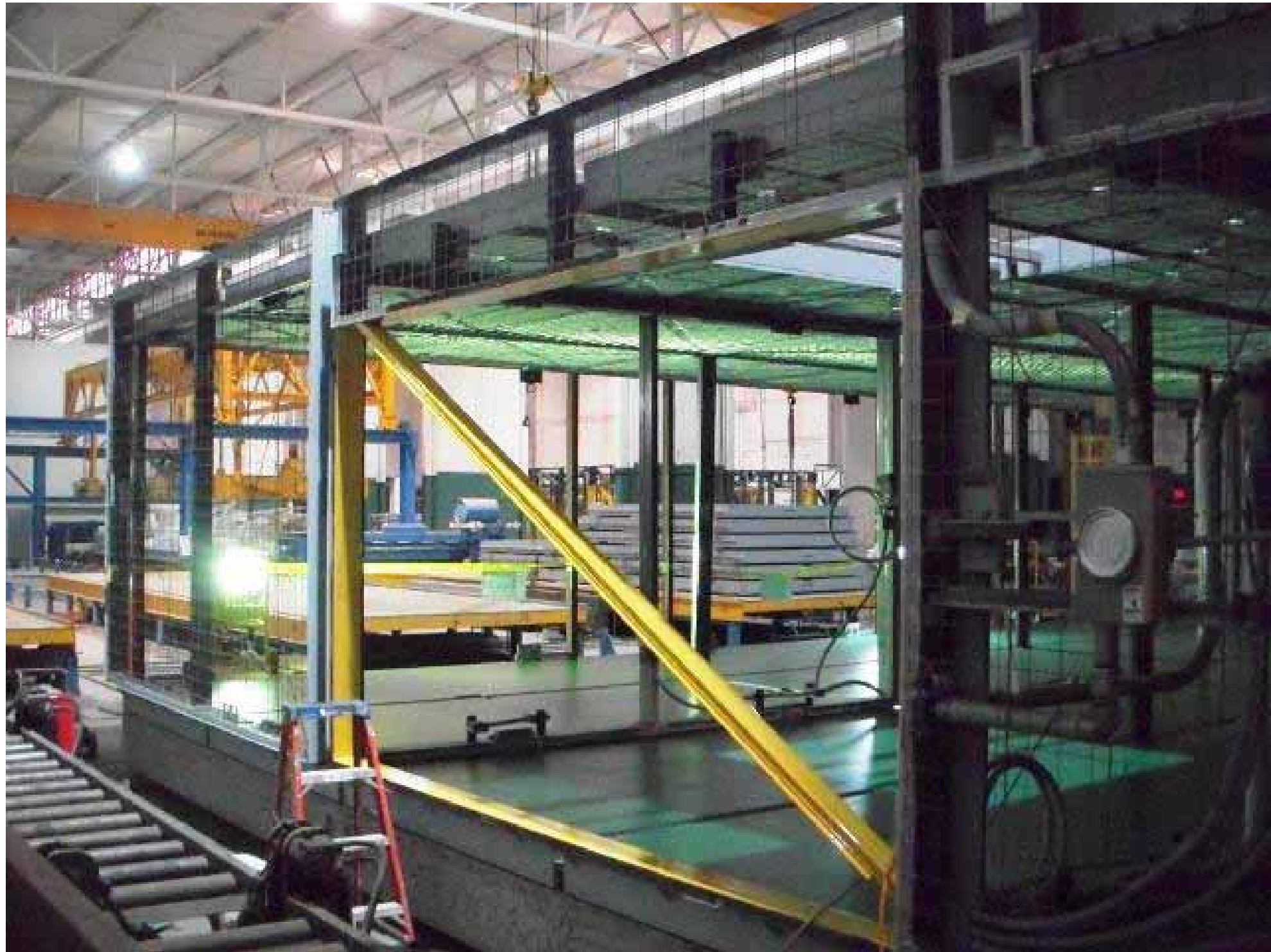
VIEW OF A LARGE WINDOW SUB-FRAME WITH TEMPORARY BRACING PAINTED IN YELLOW. THE SKYLIGHT SHOWN INSIDE WILL CREATE A NICE FEATURE ABOVE THE 3-D MODEL OF THE OPTIMA TOWERS.
